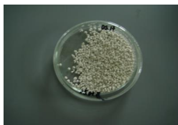
Figure 2. Granules with bacterial biofertilizers strains embedded inside
