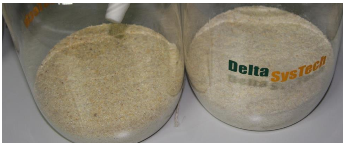
Figure 1. 300g milled corn with their own microbial load after seven days of incubation at 30°C, left -100 \mu L/air Thymus vulgaris volatile oil, right – control.
